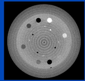
Scan with modulator, after PMSE correction
