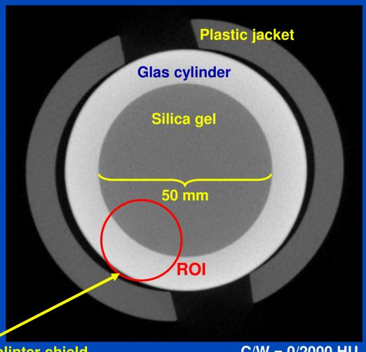
0.5 mm splinter shield (not visible in the overview scan) C/W = 0/2000 HU
