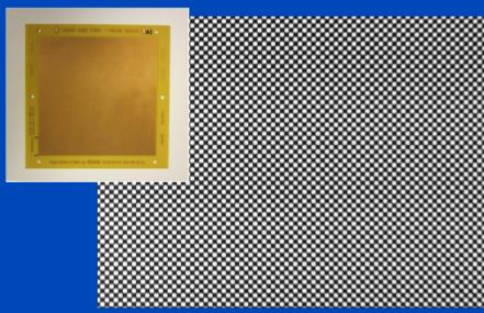
"Ideal" modulator (projection image of a copper modulator)
